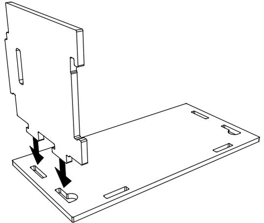
**3** Drop the other side panel tabs into the back panel slots, but **DO NOT** click the panels together yet
