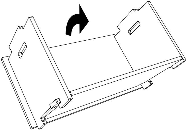
**8** Press the back panel down firmly on each side until the back panel and side panels "click" together. Repeat steps 1 through 8 to assemble the second shelf.
