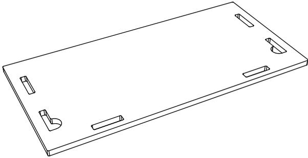
**2** Drop the side panel tabs into the back panel slots, but **DO NOT** click the panels together - the side panels need to remain loose until a later step
