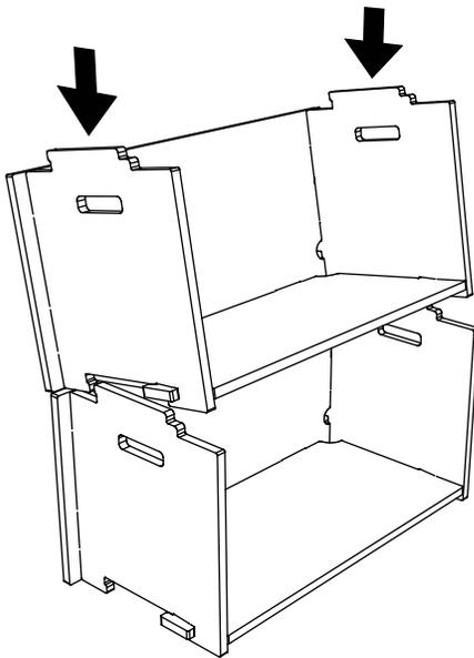
**10** Firmly pull the front of the upper shelf down onto the lower shelf to "click" it into place, locking the two shelves together. To separate the shelves, lift firmly on the front edge of the upper shelf while holding the lower shelf down.
