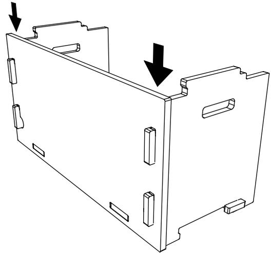
**9** Lower the back of the upper shelf onto the lower shelf, as shown
