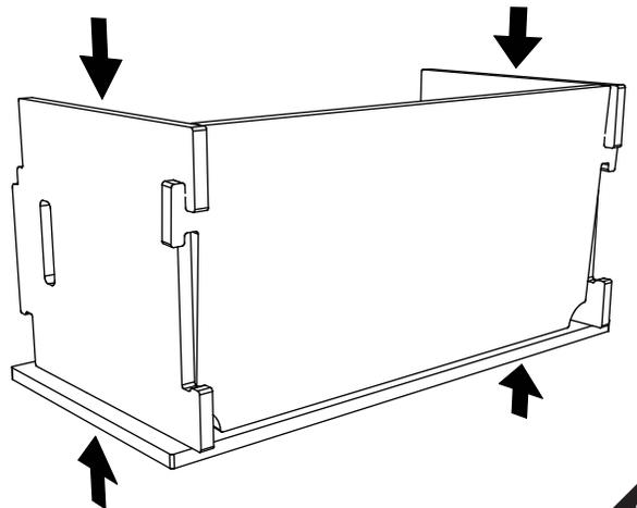
**7** Holding the back panel against the side panels, rotate the shelf forwards onto its feet
