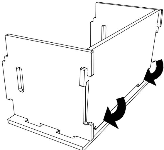
**6** Lift the back panel up on each side and hold the back panel and side panels together for the next step
