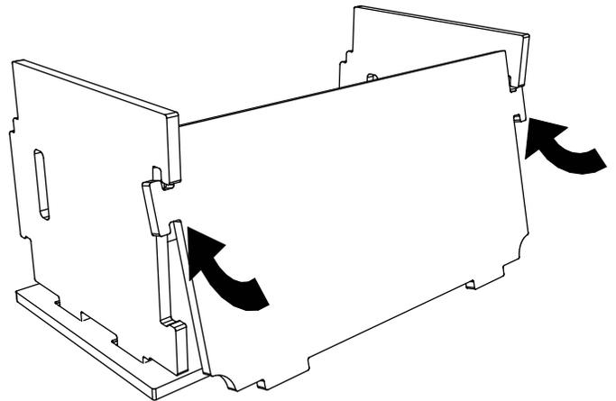
**5** Tilt the bottom panel inward so that its tabs line up with the slots in the back panel, as shown
